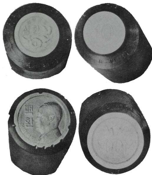
South Korean coin hubs and dies, 10-Hwan (top) and 100-Hwan (bottom), produced at the Philadelphia Mint.
